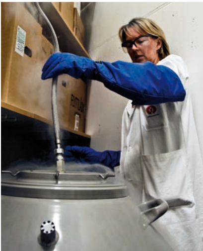
Bioengineer Liv Wenche Thorbjørnsen is making sure the liver biopsies and cells have enough liquid nitrogen in the storage tank.
